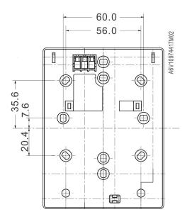
Room temperature receiver with mounting plate
